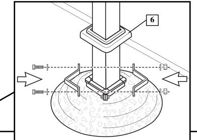
Lower clamp cover (6) over clamps and snap into proper position.
